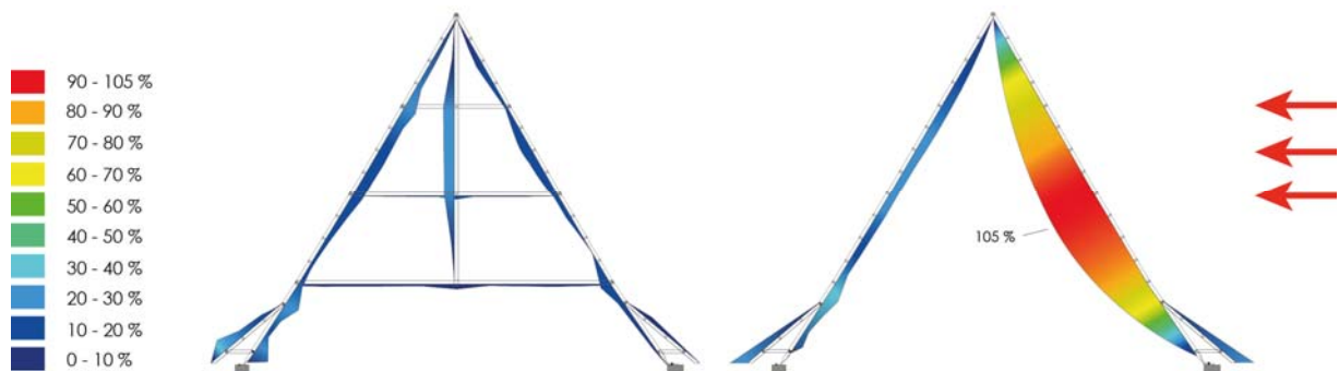
Figure 11: A pair of rafters (with and without collars) subjected to dead and wind loads: utilization in terms of effective stress (according to Batke 2015)
