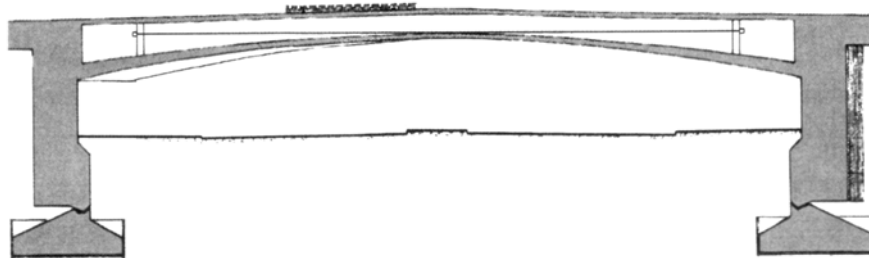
Figure 2 – The load-bearing structure of the bridge on Seidelstraße with the subsequently added external pre-stressing in the two cells of the boxes
